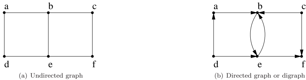
Figure 2.3: The difference between an undirected and a directed graph is indicated by drawing an arrow to show the direction.
