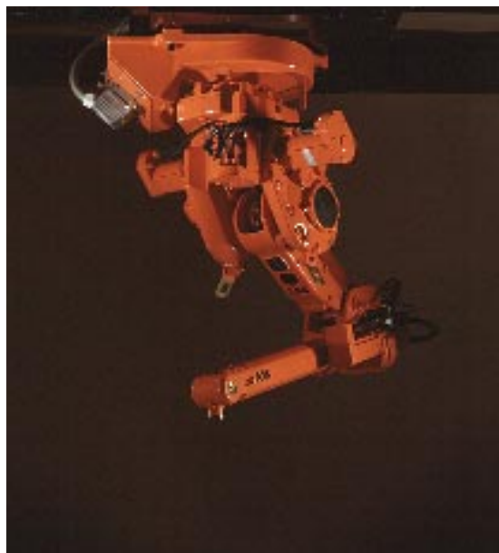
The hanging variant IRB 1400H offers high performance when floor-space is restricted, and when a large work-processing area is required.
